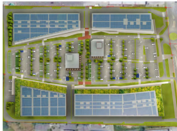
Wittenheim: 10,000 sqm of solar panels on rooftops, with a total capacity of 1.9 MW
